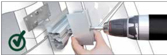
Only with a limitation to 12-14 Nm!
