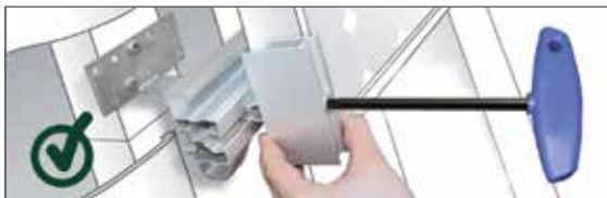
Only with a limitation to 12-14 Nm!
