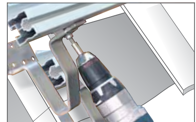
2 Hook in the rail and fasten it
